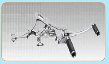
Foot controls include rear brake and gear shifter, control, driving on hills and maneuvering in city traffic.
